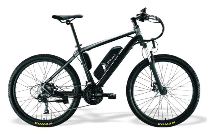
Model: 4-A M006 POWER: 350W BATERRY 48V 10.4AH SAMSUNG BATTERY Open size: 1800x630x1030mm Folding Size: 1030x1040x370mm
