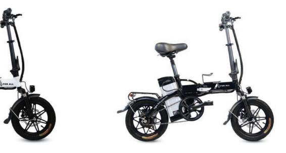
Model: 4-A CITY ELVES POWER: 250W BATERRY :48V 10AH lithium battery MAX SPEED : 40KM/H CHARGING TIME: 5-8HOUR
