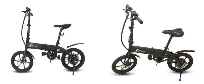
Model: 4-A A1F POWER: 250W BATERRY: 36V 4.4AH LG BATERRY MAX SPEE:D 25KM/H RANGE: 20KM
