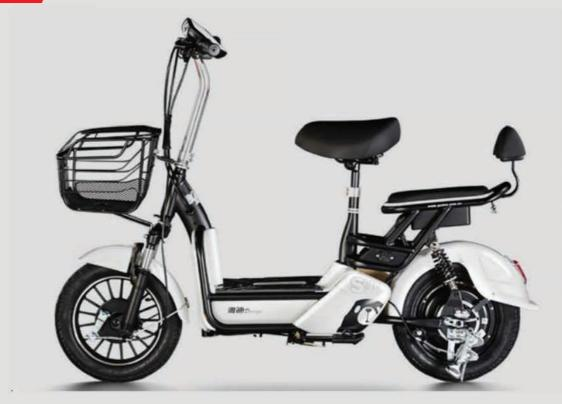
Model: 4-A XIANWANGZI POWER: 350W BATERRY 48V 12AH MAX SPEED: 25KM/H CHARGE DURATION: 6-8H
