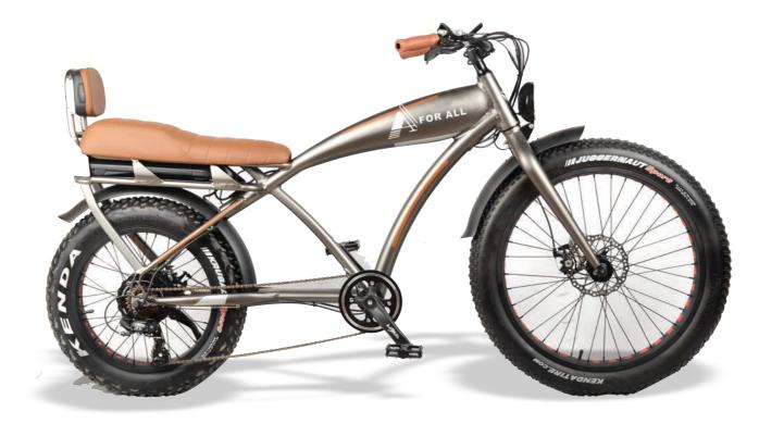
Model: 4-A E-WILD 6.0 BATERRY: POWER PACK 36V 374WH MOTOR: BAFANG FAT MOTOR CHARGER TIMES :2-5H DISPLAY: LCD METER
