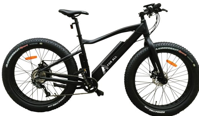
Model: 4-A E-WILD 50S 4-A BATERRY: POWER PACK 36V 374WH MOTOR: BAFANG FAT MOTOR NET WEIGHT: 24.7KG CHARGER TIMES :2-5H DISPLAY: LCD METER FRONT LIGHT: OPTIONAL MAX RANGE: 35-45KM
