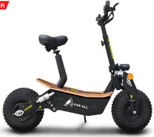
Model: 4-ALL MONSTER POWER: 2000W BATERRY:48V 12AH LEAD ACID BATTERY WEIGHT: 50.8 KG MAX SPEED: 50KM/H CHARGE TIME : 5-8 HOURS
